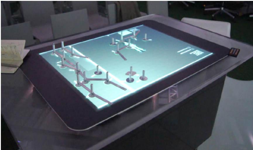
Figures 4.10 & 4.11: Virtual reality design tool for the development of flexible ceiling mounted systems for operating rooms: a touch table with tangible configurable system pieces and large screen displaying the operating room with the created system (photos by student Sanne-Marye Huijing during her Industrial Design Engineering Master assignment at University of Twente)
